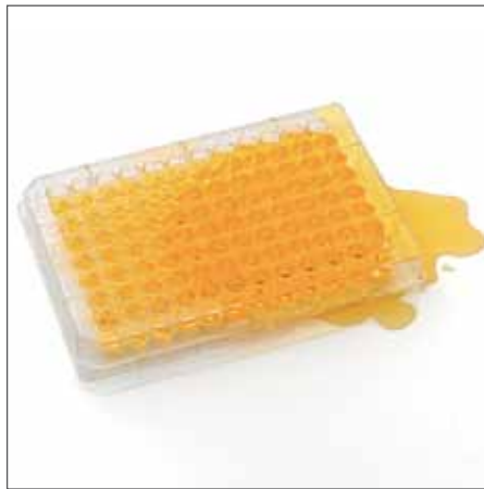
Spilling of plate caused by clogged needles
